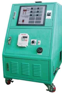
Main Hot Melt Machine
